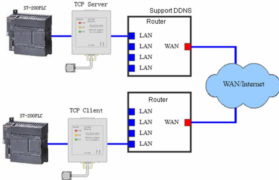
Two pcs S7-200PLC can achieve remote communication on the Internet via the ES-ETH-PPI, you need a router which supports dynamic domain name (DNS),in order to avoid the high cost of fixed IP address from the local telecom, and this router is very common now, please notice the instructions on the package when you purchase it.
