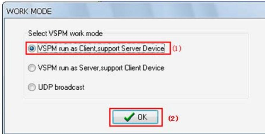
Add a virtual serial port, the remote server IP address = ES-ETH-PPI IP address, remote server monitoring port = ES-ETH-PPI port.
