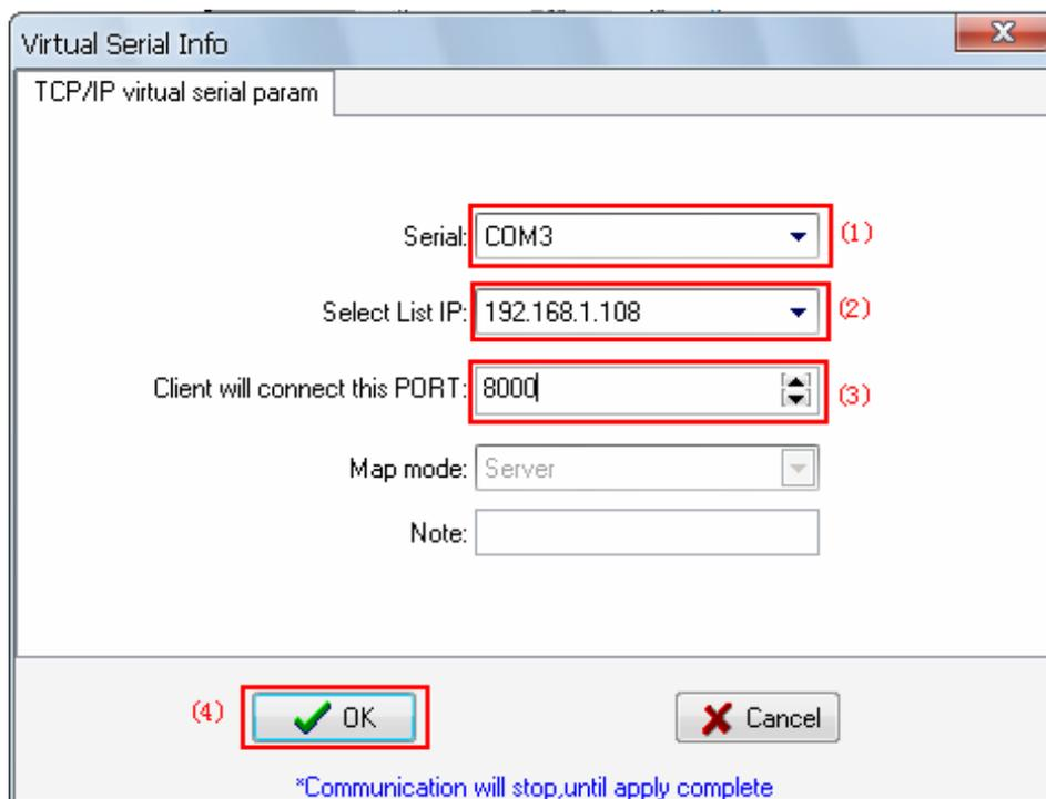
Click OK and exit the software and re-run VCOMM, server side VCOMM will accept as many as client side ES-ETH-PPI connections, and it's unlimited. A new serial port COM3 will appear on the PC after the connection is established. And this serial port will also appear in the Windows System Device Manager, then you can choose this serial port in your applications,like STEP7 Micro/WIN.
