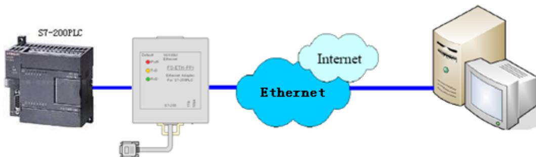
Set the ES-ETH-PPI network parameters, the gateway of ES-ETH-PPI, PC and router must be same, the DNS server needn't to be setted because you don't use the dynamic domain name on the Internet.
