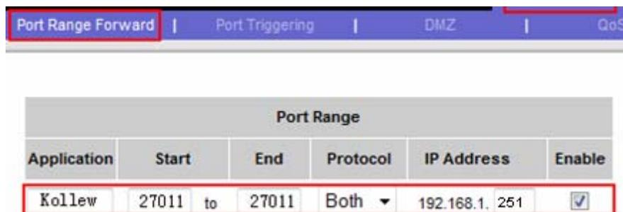
The server port = local port of server ES-ETH-PPI; IP address = IP address of server ES-ETH-PPI; Select the "Enable", click "Save" button to save these configured parameters.
