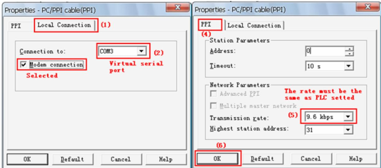
Click the "Communication" button to enter the communication settings, double-click "connection" to set the modem parameters.
