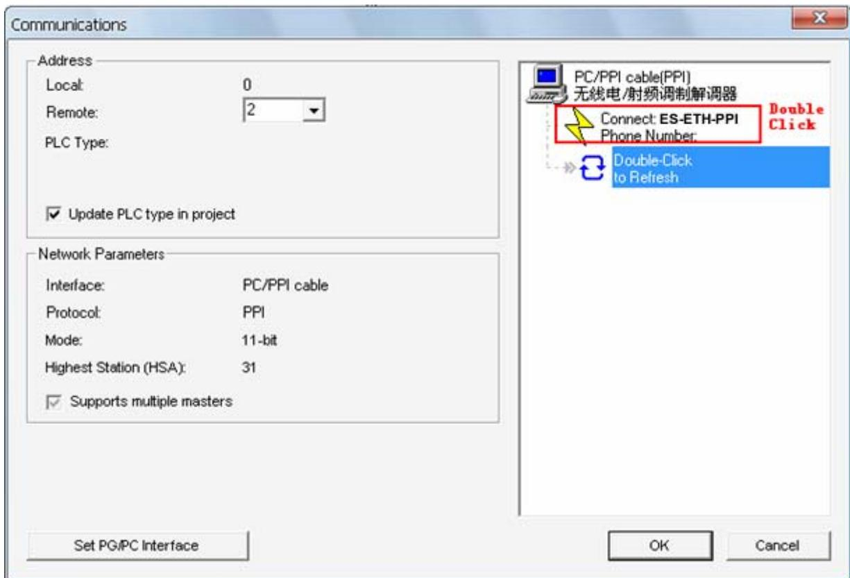
Select the "Radio / RF modem" and configure serial port parameters, choose no parity 10 bit mode.
