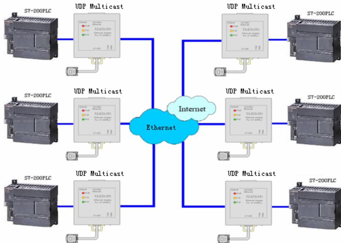
When multiple S7-200PLC need to exchange data each other, of course UDP multicast mode is the best working mode. Using UDP multicast can directly replace the original multi-point RS485 communication. But please notice that at this time the ES-ETH-PPI only supports S7-200PLC free port RS485 communication mode, do not support PPI,advanced PPI,Multi-master PPI communication protocol and MPI and profibus protocol.
