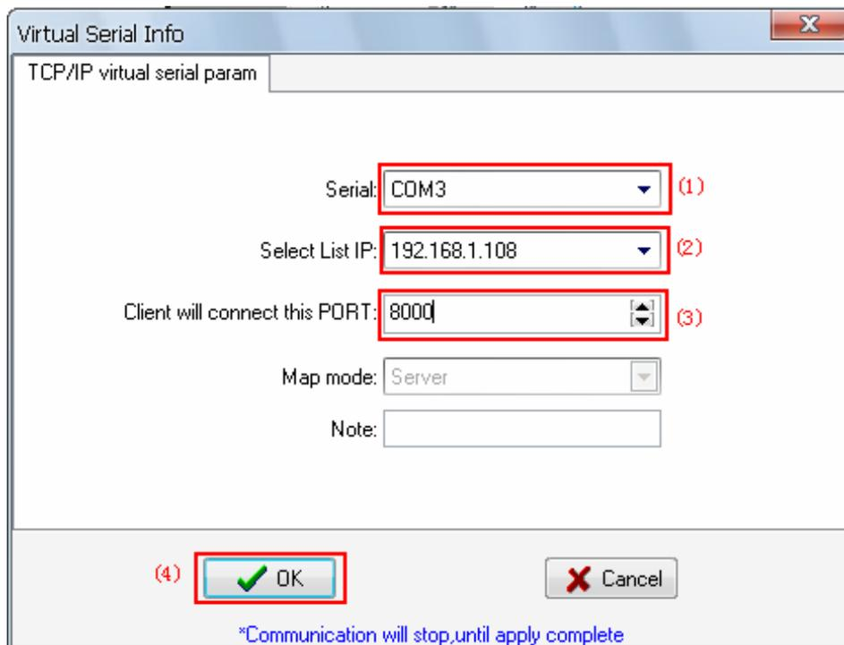
Click OK and exit the software and re-run VCOMM, the server VCOMM will wait the connection of client ES-ETH-PPI, then it will create a new serial port COM3 after establishing the connection, and it will appear in the Device Manager of the Windows system, then you choose this serial port in your application software, such as STEP7 Micro/WIN.
