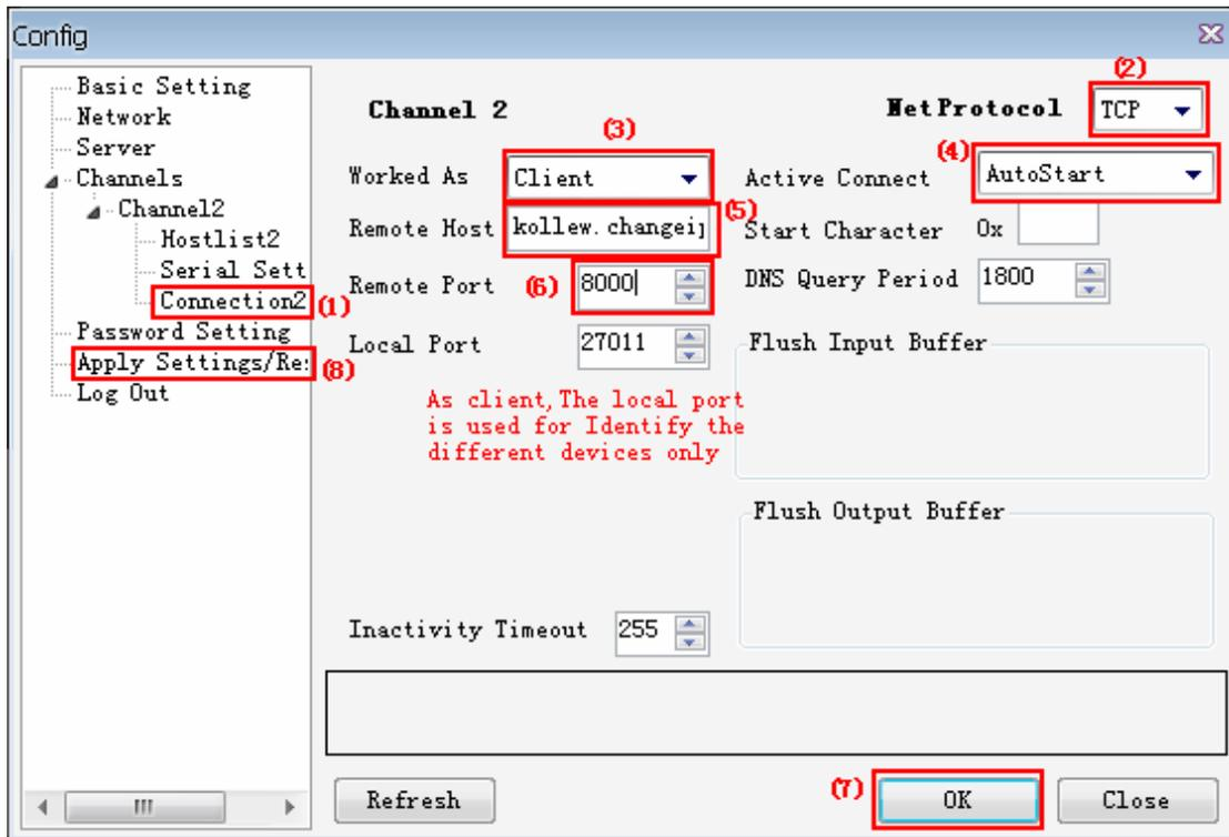
Input the IP address of the router in the IE browser address bar of the remote PC and then appear the router setting interface, set the port simulation for PC, as shown below. If your PC does not use the router to access Internet, then this step can be omitted.
