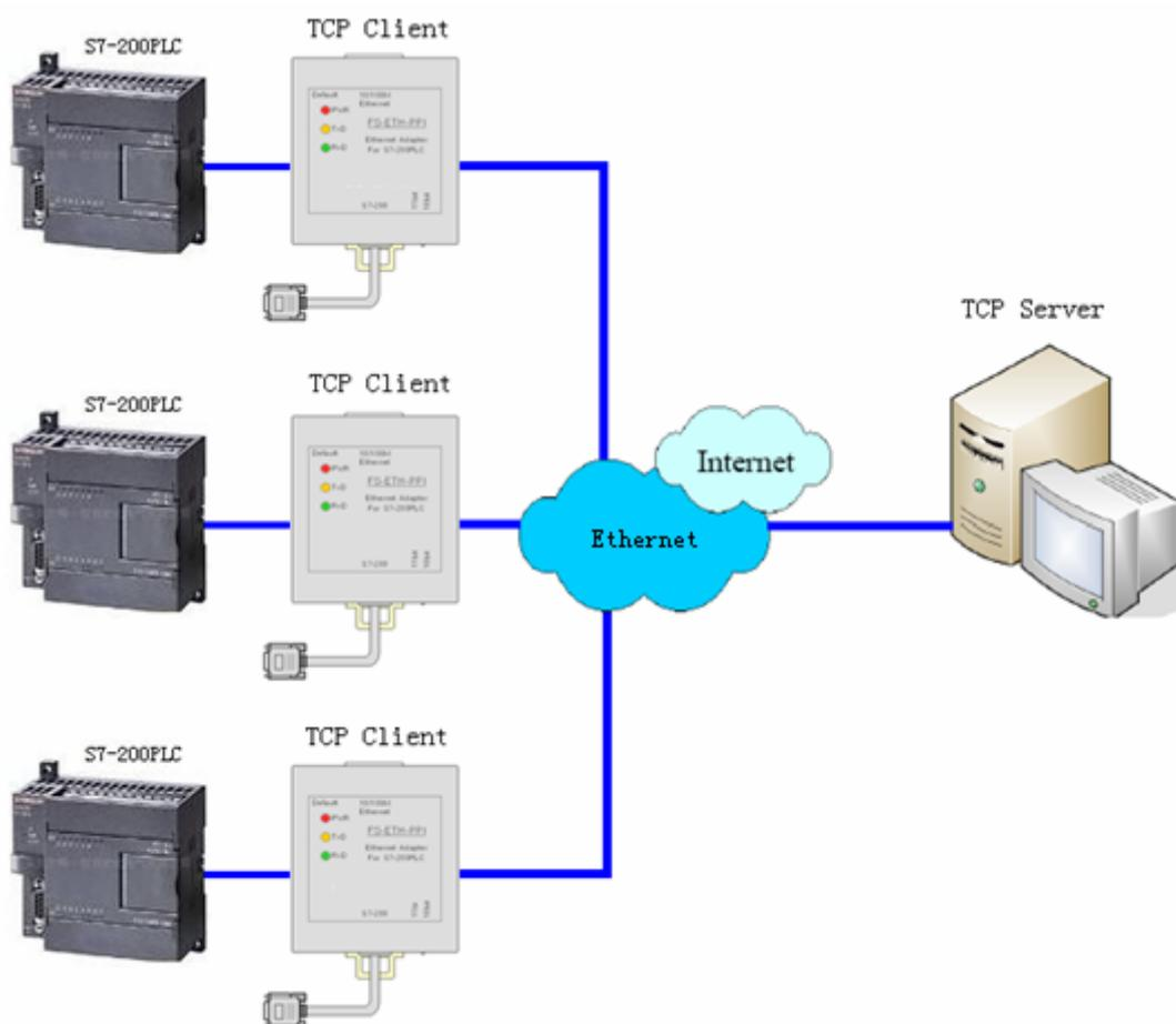
When multiple PLCs communicate with a PC via Ethernet, you need to set every ES-ETH-PPI connected with PLC as TCP Client, set the PC as the TCP Server, let every client ES-ETH-PPI takes initiative to connect the server PC. When VCOMM Virtual Serial Port Software work as TCP Server, it allows unlimited number of connected clients.
