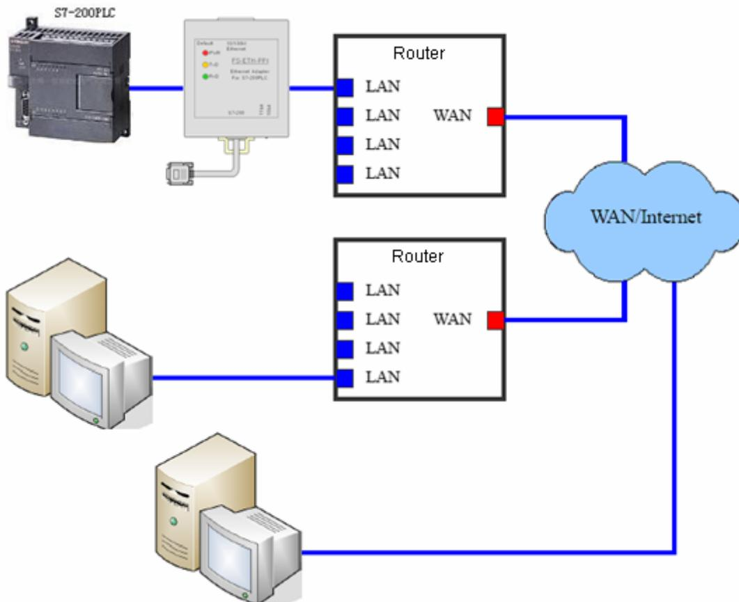
The most economical way to achieve the remote communication in the Internet between the PC and S7-200PLC is that set the ES-ETH-PPI as the client, set the PC as the server, install and run the DDNS software on the PC, and set the port mapping for PC on the router of PC side. As shown below:
