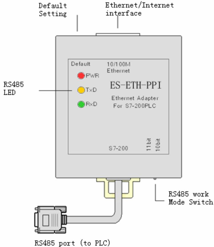
Ethernet interface: Standard RJ45 socket, automatically adapt 10M/1000M Ethernet .Use the standard network cable, not crossover cable whether you connect the switch or directly connect the PC.
