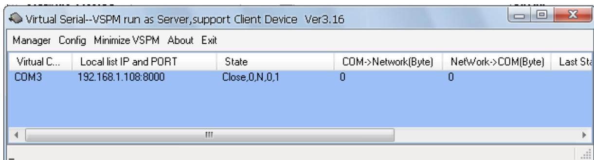
You can also set the ES-ETH-PPI as the server, set VCOMM as the client, but the router connected with ES-ETH-PPI need to have the DNS function, or you can use a PC connected to the router which is connected with the ES-ETH-PPI to run the peanut shell software to resolve the domain name. When the VCOMM software work as the client, you also could input the domain name directly in the remote server IP address, support DNS resolution.
