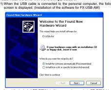
Insert the included CD-ROM into the personal computer's CD-ROM drive Click [ Next > ]. The installation of the FX-USB-AW software will begin. - If using Windows<sup>®</sup> 98, Windows<sup>®</sup> 98SE, Windows<sup>®</sup> Millennium Edition, and Windows 2000, A window solect the location of the installation files. Please select the CD-ROM drive.
