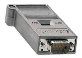
PB BUS CONNECTOR WITH AXIAL CABLE OUTLET F.INDUSTR. PC, SIMATIC OP, OLM; TRANSMISSION RATE 12 MBIT/S; TERMINATING RESISTOR WITH SEPARATING FUNCTION, METAL HOUSING
