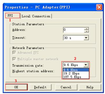
4. After the USB/MPI+ V4.0 connect the USB port of computer and PPI interface of S7-200 PLC, click the "Communications" button in the main interface and then double click "Double-Click to Refresh" icon, then can find the PLC. Choose this PLC and click "OK" button to return the main form.
