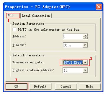
4. After the USB/MPI+ V4.0 connect the USB port of computer and MPI interface of S7-300/400PLC, click the following red circled button in the "SIMATIC manager". If it appears the red squared data, it shows the online test is OK. Now the setting is finished.
