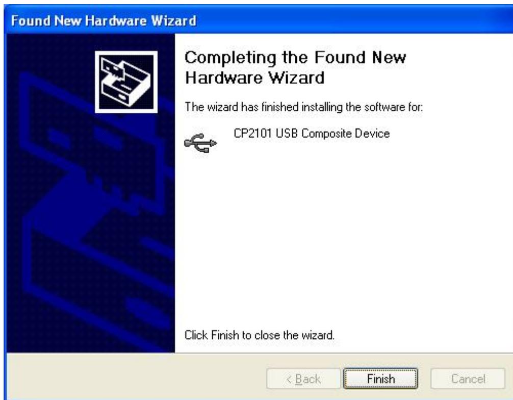
6. After setting up, please make sure the "port (COM and LPT)" of "Start \ Settings \ Control Panel \ system \ hardware \ Device Manager" appears "CP2101 USB to UART Bridge Controller(COMx)". This COMx is the COM message of the USB programming cable. From then on, as long as you insert
