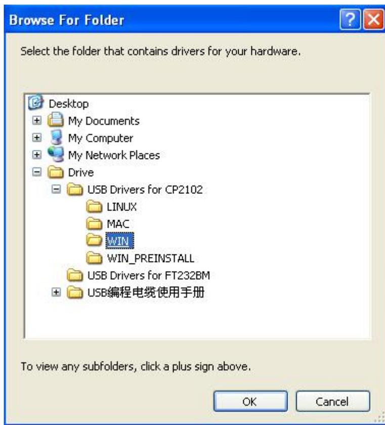
3. Windows will detect the setting information, and load the driver to install.
