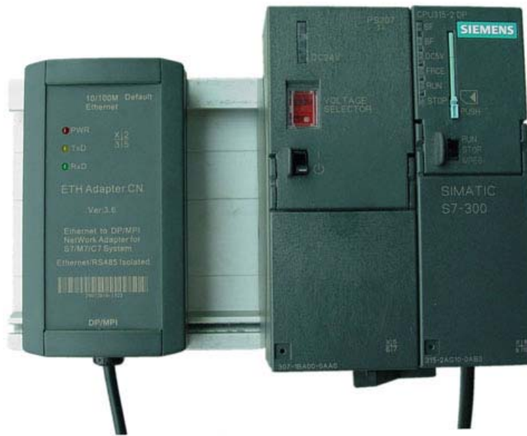
ETH Adapter CN adapter has been installed on the S7-300PLC rail
